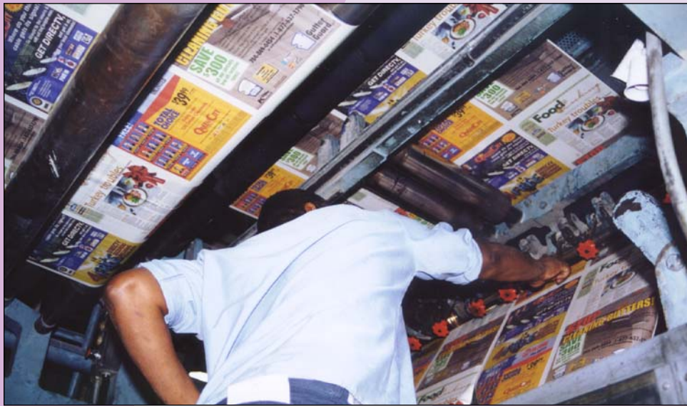
The Charlotte Observer uses a MAN Roland FLEXOMAN press to print 300,000 copies of the newspaper a day.
